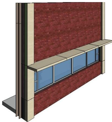
Fig 12: Exterior View of Panel Assembly with Overhangs
