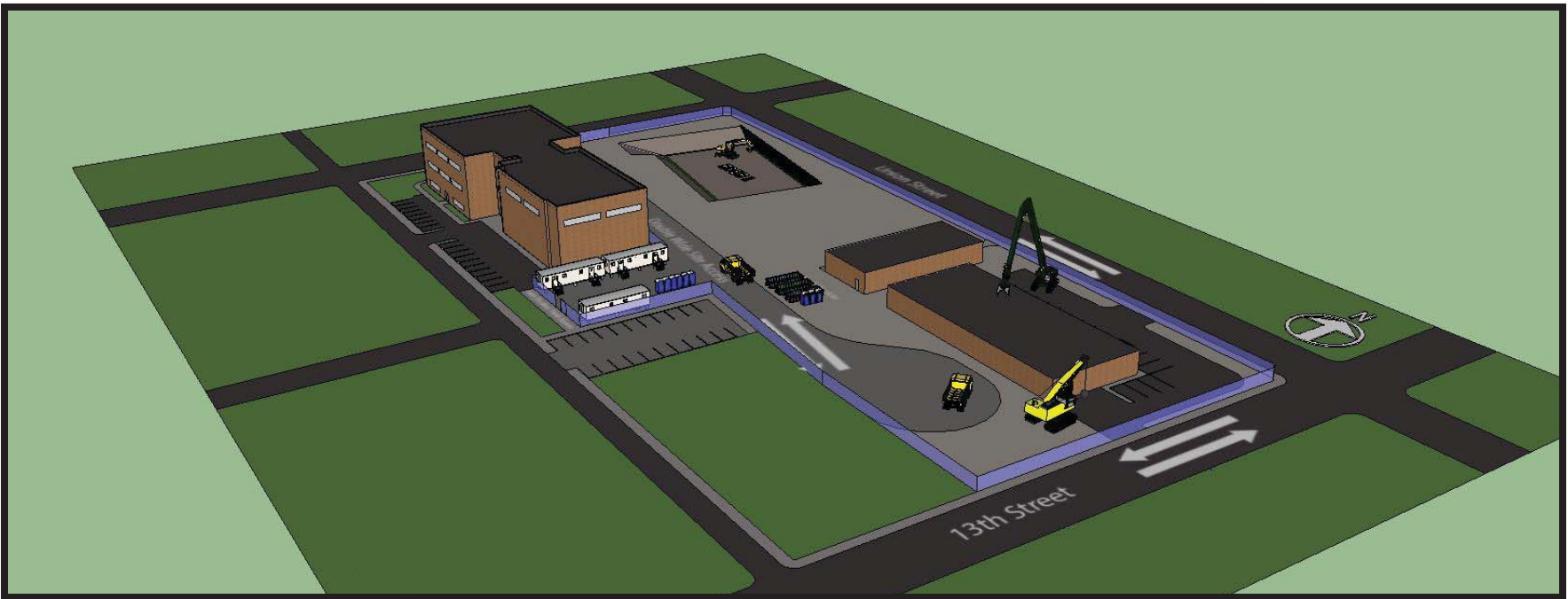
Demolition Logistics Plan
